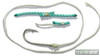
Hook line, nylon 3mm \varnothing .
